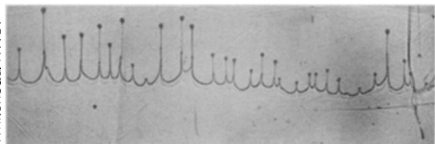
Whitehead demonstrates how a thin line of a water-glycerin mixture injected into a more dense glycerin bath develops periodic instabilities after 45 seconds. Each plume represents molten rock ascending toward a magma chamber.
