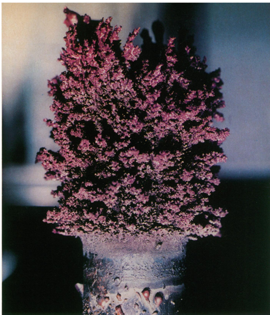
Uranium deposited on negative electrode at end of electrorefining phase of fuel reprocessing. Colorless chlorides of lithium and potassium comprise 97 percent of crystal; remaining 3 percent uranium chloride imparts amethyst hue. Electrorefining is the only IFR technology not yet proven on demonstration scale.
