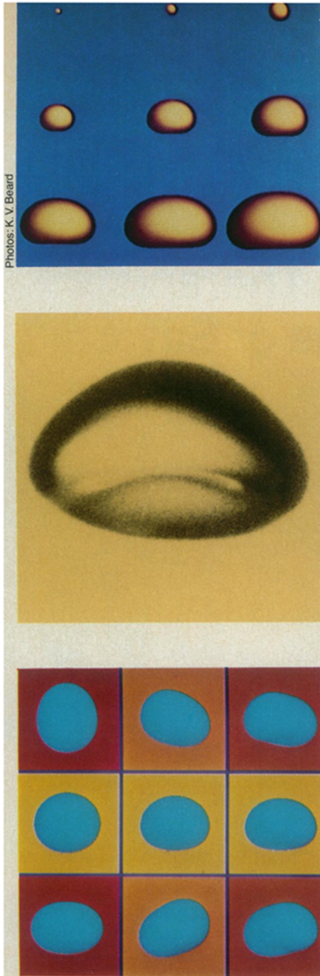
Larger and larger raindrops look more and more like hamburger buns, as shown in the top, computer-generated sequence of images. The middle photograph captures a giant water drop, about 8 millimeters across, suspended in a wind tunnel’s airstream. In the next sequence of images, third from top, each column illustrates the preferred oscillation shapes for drops of a particular size, ranging from 2 mm in diameter on the left to 6 mm on the right (not drawn to scale). The strip, below, shows the rotation of one raindrop oscillation shape.
