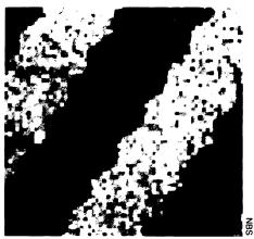
surfaces of single crystals of iron mixed with 3 percent silicon. The illustration above shows magnetic domains in a section of the crystal surface 50 by 50 microns. The difference in polarization between light and dark domains is approximately 60 percent. The best resolution of detail so far achieved with the device is 50 nanometers, a limit imposed not by electron characteristics but by vibration of the stage on which the sample rested.
