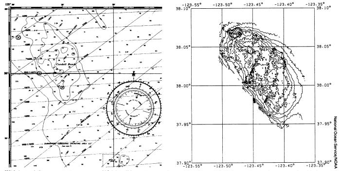
With its multibeam mapping systems, NOAA will be able to produce contour maps of seafloor topography in considerably better detail than most existing charts. Here, for example, the Cordell Bank off the northern California coast has been mapped with conventional techniques (left) and by a multibeam mapping system (right). NOAA plans to produce bathymetry maps with depth contour intervals of about 20 meters at a scale of 1:100,000.
