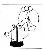
The Space Ball, which is made in Taiwan, runs on a 9-volt battery hidden in the toy's base. This activates an electromagnet that, in turn, "kicks" another electromagnet in the lower ball. "Basically, it's a very efficient electric motor," says Wolf.
