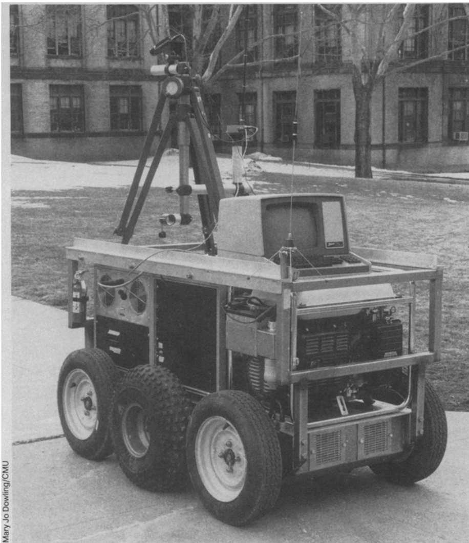
Carnegie-Mellon's Terregator is an outdoor vehicle used in navigation research.
