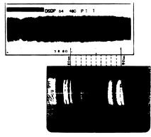
MRI compared with X-rays of an ocean core sample: MRI (bottom) distinguishes between richly organic layers (light bands) and layers that contain little organic material (dark bands).
