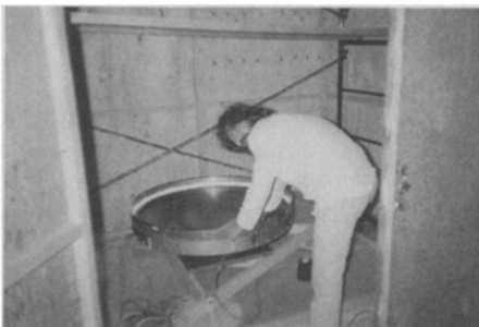
Astronomer Mario Beauchemin checks position of prototype liquid mirror underneath the scaffolding that holds the telescope camera.
