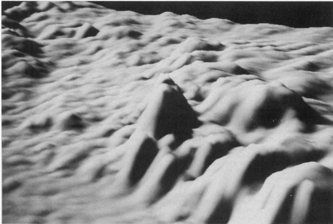
Using NOAA's raw data tapes, Kruse and Schmieler have generated computer images that have the highest resolution of any seafloor images produced in the Exclusive Economic Zone mapping program. The smallest feature that can be resolved in this image is 4-by-4 meters in size. The pinnacle in the middle of this picture was discovered when the researchers processed the sonar soundings. It is the second-highest peak on the Cordell Bank, measuring 100 feet tall and reaching to 120 feet below the ocean surface.
