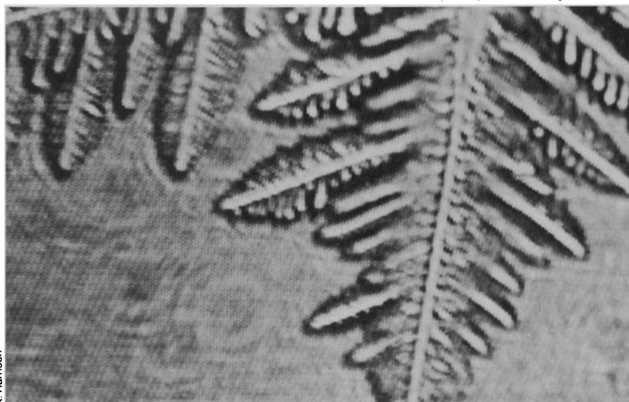
Ice crystals, when free to grow in pure water, normally create dendritic patterns.
