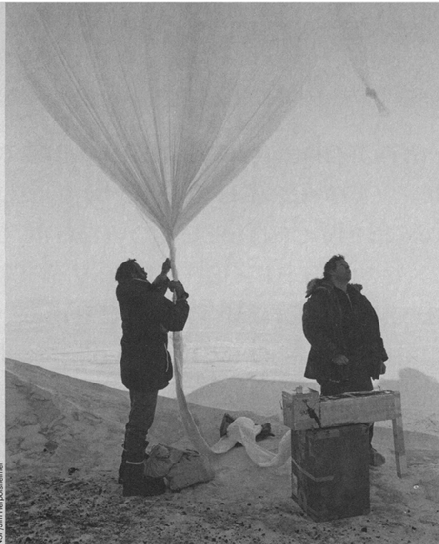
NOZE scientists prepare a balloon for atmospheric measurements in Antarctica.
