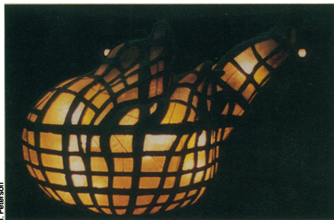
The Statue of Liberty's original torch and flame, shown here, had to be replaced because of extensive corrosion damage. Holes cut into the copper flame to create windows allowed moisture to leak into the statue's arm. The original torch is on display in the museum.
