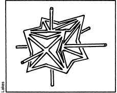
So far, Lakes has found ways to make these "reentrant" foams, as he calls them, from polyester, silicone rubber and even copper metal. In the case of polymers, the method involves squeezing the material while it's hot, then cooling it to freeze in the required structure.
