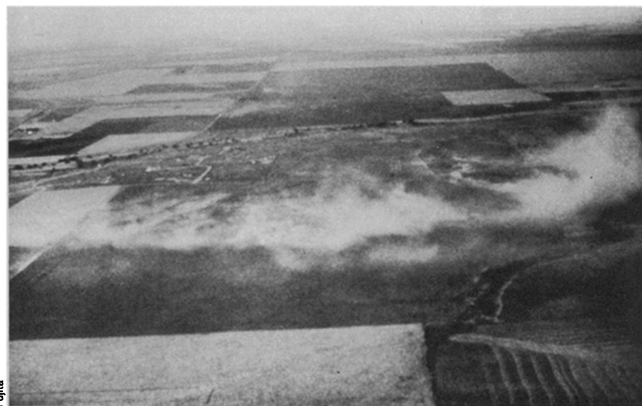
In the high plains near Denver, shown here, the precipitation associated with the downdraft often evaporates before the downdraft hits the ground. In such cases, a ring of spreading dust is sometimes the only clue that a microburst exists.
