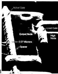
With careful engineering, including the use of electron-beam lithography for delineating device features, IBM researchers have shown that high-performance, low-temperature silicon transistors with key parts smaller than 0.1 micron can be fabricated.
