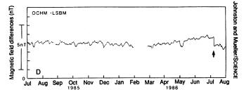
The subtle increase of field strength between March 1986 and the quake (arrow) is visible in the magnetic record, but it may be indistinguishable from background noise.
