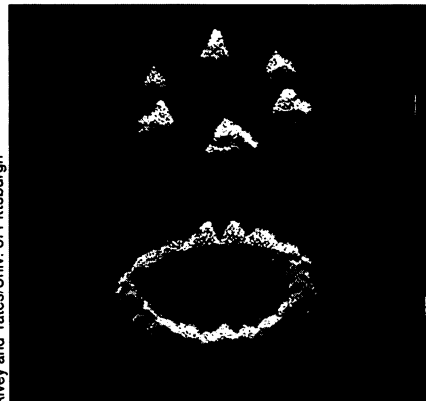
With ESDIAD, the six fluorine ion beams indicate that at 85 kelvins, \text{PF}_3 molecules are sitting with their fluorine atoms sticking up in the air and are oriented in two possible positions over the underlying nickel crystal (top). As the temperature increases to 275 kelvins, the fluorine beams spread out into a ring, indicating that the molecules are spinning around their phosphorus hubs (bottom).
