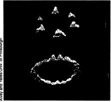
With ESDIAD, the six fluorine ion beams indicate that at 85 kelvins, PF<sub>3</sub> molecules are sitting with their fluorine atoms sticking up in the air and are oriented in two possible positions over the underlying nickel crystal (top). As the temperature increases to 275 kelvins, the fluorine beams spread out into a ring, indicating that the molecules are spinning around their phosphorus hubs (bottom).
