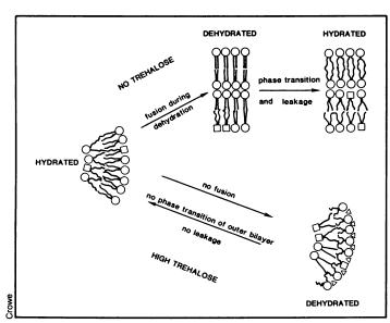
Liposomes are damaged when dried and then rehydrated, because the membranes fuse together and undergo a phase change. Both fusion and phase changes can cause membranes to leak. However, sugars (small triangles at lower right) lodge between the lipids in the liposomes, preventing both fusion and phase changes.
