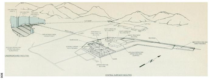
A home for more than 10,000 years: Located 1,000 to 1,500 feet below the top of Yucca Mountain, the underground grid of disposal rooms (shown in cutaway) will be the final resting place for high-level waste from nuclear power plants and nuclear weapons construction. The temporary surface facility will sit on land to the east of the mountain. As part of the characterization process, the DOE will start drilling the first of the two exploratory shafts (cutaway) in June of 1989.
