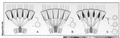
Above, two compound-eye models, seen here from the side, either use just one type of cylindrical lens (A) or lack lenses altogether and simply rely on reflection to focus light (B). But the parabolic superposition eye (C) uses a collection of lenses and light-reflecting structures. As shown in the cross-section photomicrograph at right, the newly discovered eye contains cylindrical lenses held inside crystalline cones.
