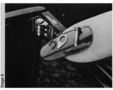
The solution was to coat threads on both bolts and nuts with a thin layer of Teflon. The coating prevents paint and primer buildup and easily survives the high-temperature primer bath without contaminating the liquid.
