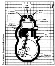
Automobile makers use a complex array of moving parts - valves, rocker arms and rods - to make the powerful "four-cycle" engine, which combusts fuel on every fourth stroke of each piston. The "two-cycle" engine, on the other hand, does without those mechanisms. And although it is notorious for slurping fuel and exhaling a blue-smoke miasma of unburned fuel and oil, the twocycle's simple design still makes it desirable for lowpower use in lawnmowers,
