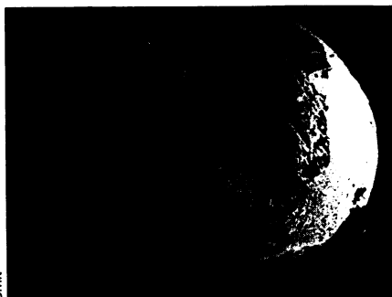
Clinopyroxene crystals suggest this spherule was formed by impact of extraterrestrial body with Earth. Scale bar is 42 microns.
