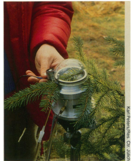
Transpiration and photosynthesis recorded in spruce branches. Such field data helped show that needle symptoms in declining trees were not a direct effect of air pollutants.
