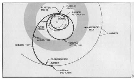
Galileo's route to Jupiter is called VEEGA, for Venus-Earth-Earth-gravity-assist. The craft's roundabout flight path, which first carries it inward to make it go out, will rely on the gravitational influences of other solar-system bodies to accelerate and re-aim Galileo toward Jupiter.
