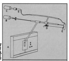
Diagram (not to scale) depicting a European robot bee (E) and its \$125,000 "life support" system. A computer-programmed recorder (A) controls the model bee's figure-eight dance pattern; a step motor (B) makes the model's body waggle; another step motor (C) connected to a syringe (S) pumps scented sugar water through plastic tubing as an offering to nearby begging bees; while an electromagnetic driver (D) vibrates the model's "wing."
