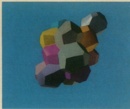
The "Voronoi cell evolver" program divides space into a jumble of polyhedrons, then rearranges the boundaries between the shapes to minimize the total surface area of the interfaces.
