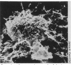
Scanning electron micrograph of the interior surface of a plastic pipe after exposure to Pseudomonas-infected water. The bacteria secrete a sticky material that adheres to pipe walls and forms a shield against disinfectant treatment.
