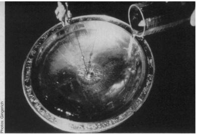
Schissler's 16th-century sundial. A bead on a string stretching from the bowl's center to a figure on its rim casts a shadow on the calibrated inner surface. Pouring water into the bowl shifts the bead's shadow by 10° to 20°, in effect turning back time.
