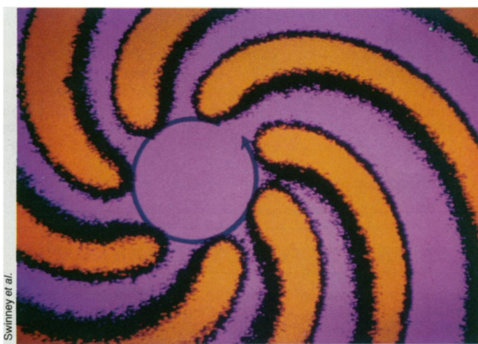
Pinwheel pattern depicts a spiral arm rotating within a gel hosting reactions of malonic acid, potassium bromide and potassium bromate. Scientists created the image by superimposing a spiral arm's position at 2-minute intervals. Though its shape remains constant, the arm's location changes, ruling it out as a Turing pattern.
