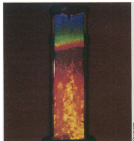
In this layered colloidal polycrystal, consisting of polystyrene spheres immersed in water, different colors correspond to different sphere spacings.
