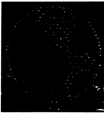
Arguably the smallest map of the Western Hemisphere, the actual diameter of this image — greatly enlarged here — measures about one-fiftieth that of a human hair. Each dot is a mound of gold containing thousands of atoms.
