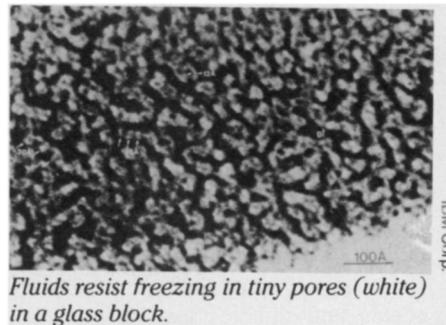
Fluids resist freezing in tiny pores (white) in a glass block.
