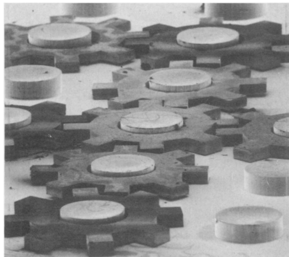
By placing nickel microgears on nearby shafts, engineers have assembled what may be the smallest metallic gear train ever made.
