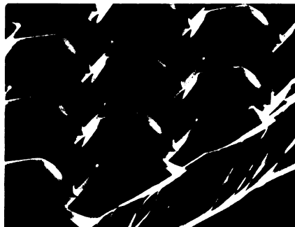
Micrograph shows the rounded, mushroom-like structures that interlock when two such sheets are pressed together.
