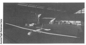
Perseus gets its push from a propeller on the tail of the plane, allowing scientific instruments onboard to sample clean untainted air through a hole in the nose.
