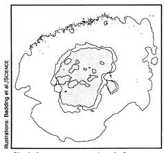
Shaded area represents iron before compression. Squiggly line just beyond the shading shows how much the sample swelled when squeezed together with hydrogen. The gas itself extends to the outermost border.
