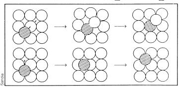
An atom deposited on a surface can move either by "hopping" an energy barrier to get from one location to another (bottom) or by trading places with a substrate atom (top).
