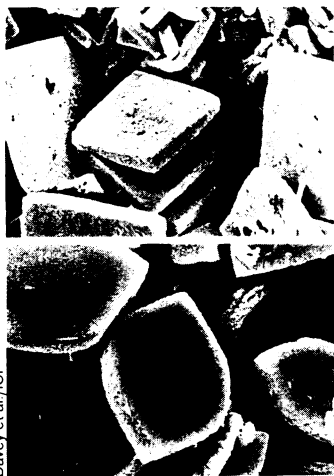
Phosphonate compounds cause rhombic barium sulfate crystals (top) to develop curved sides (bottom).
