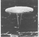
shaped semiconductor lasers measuring 2 to 10 microns in diameter. Commercial semiconductor lasers, such as those used in compact-disk players, typically meas-
