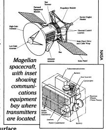
Since the craft has a limited capacity to store radar data, the transmission failure forced NASA scientists to halt radar studies until Magellan resumed full communication with Earth. (Despite the equipment problem, the craft could still receive electronic signals critical to maintaining its proper orbit around Venus, Okerson notes.)
