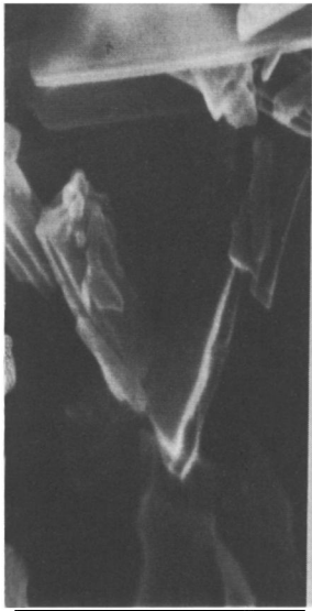
Pure taxol crystals as seen through a scanning electron microscope. To get the crystalline form, chemists must work with a crude extract taken from the bark of a yew tree.
