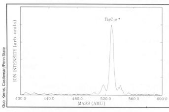
A readout from a mass spectrometer shows that a reaction between titanium and methane has produced a relatively large number of molecules — all with a mass of 528 atomic mass units.
