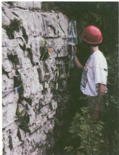
Looking like a tree surgeon with her patients, researcher Sarah Owen checks on an innovative cliff-side sprinkler system constructed from hospital intravenous feeding equipment.
