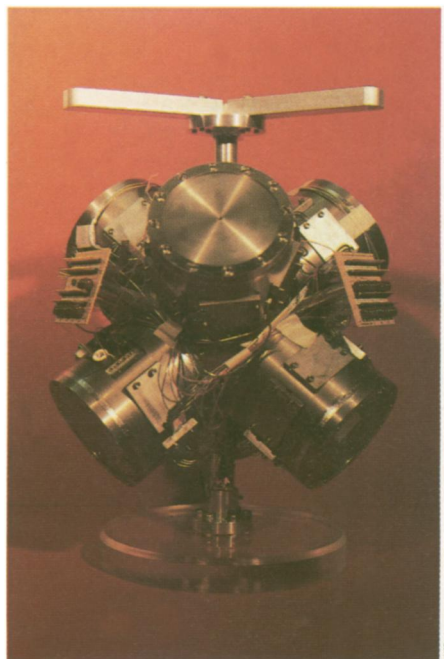
The three mutually perpendicular arms of this gravity gradiometer contain sensitive mass-spring motion detectors.
