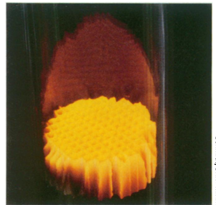
Methane oxidation causes porous catalytic plug's golden glow.
