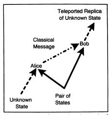
Using quantum teleportation via a pair of EPR particles with correlated quantum states to convey a particle's unknown quantum state from Alice to Bob.
