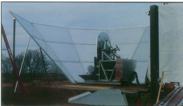
Above: Python, a radio telescope at the South Pole, searches for temperature fluctuations in the microwave background on the angular scale of 2.8^\circ . Left: At Saskatoon, Saskatchewan, an instrument called BigPlate looks for hot and cold spots in the microwave background at an angular scale of 2^\circ . Below: A balloon experiment, the Microwave Anisotropy Experiment, searches for temperature fluctuations on the 0.5^\circ scale — roughly the width of the full moon as it appears on the sky.
